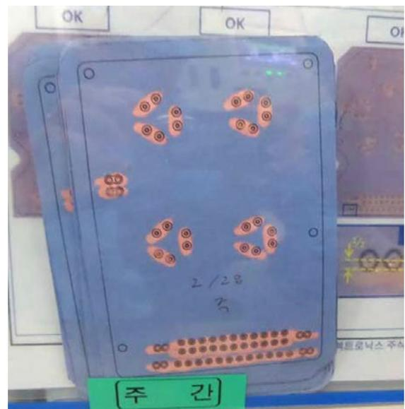
Figure 5: Flux spreading visual check. Solder joint positions are printed on the check paper. Visual criteria are stored at the machine.
