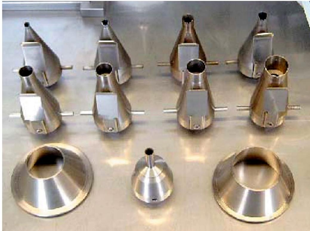
Figure 3: Some of the soldering nozzles that are typically used in the selective soldering process.
