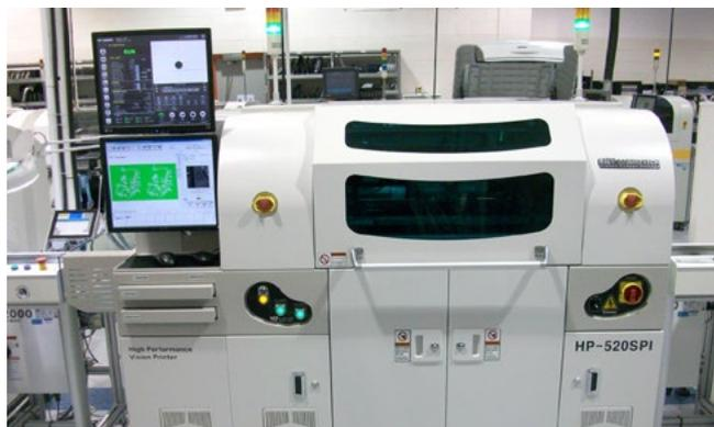
With the new screen printer, Etratech's manufacturing team went from receiving process indicators at the end of the line to the new printer actually being able to make adjustments on-the-fly in real-time.
