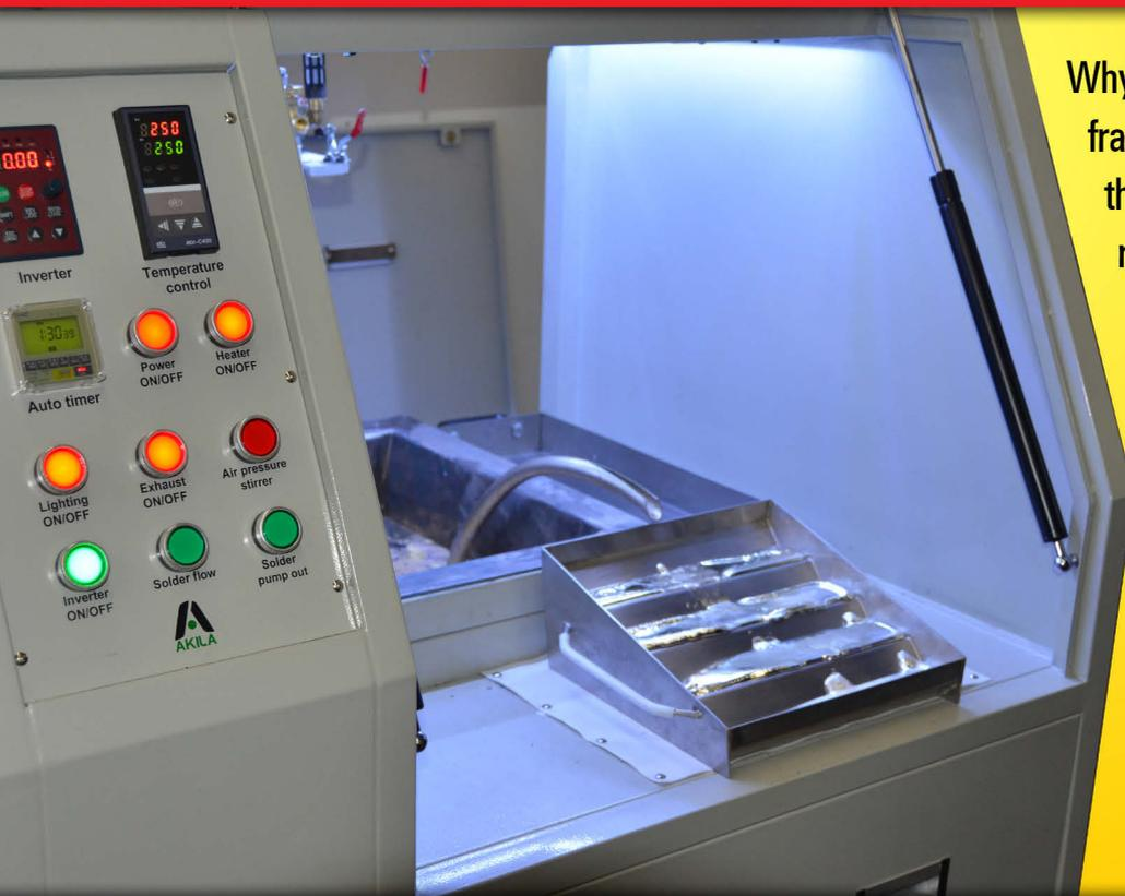
Why sell your dross to a recycler for a fraction of its true value? Ask us about the new compact Akila off-line solder recovery unit that, along with our MS2® Molten Solder Surfactant, takes the guesswork out of the solder recovery process.
