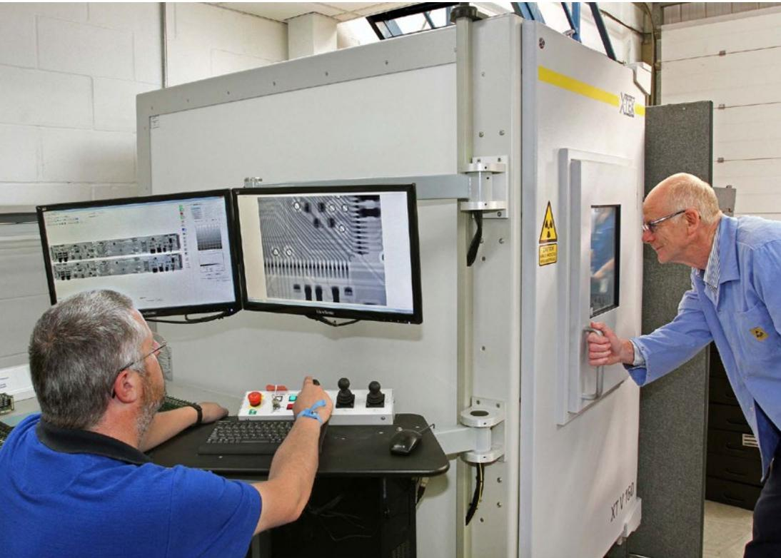
Figure 2: X-ray capability is something to look for in a higher-end rework/repair facility.
