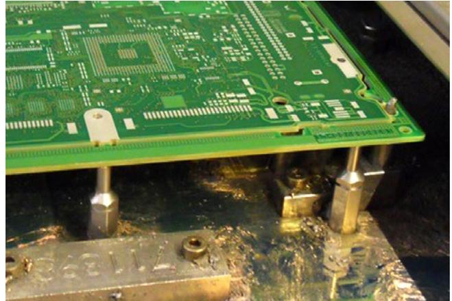
Figure 14: Pins on the multi wave plate serve to flatten the board and the slotted pin to position the assembly.
