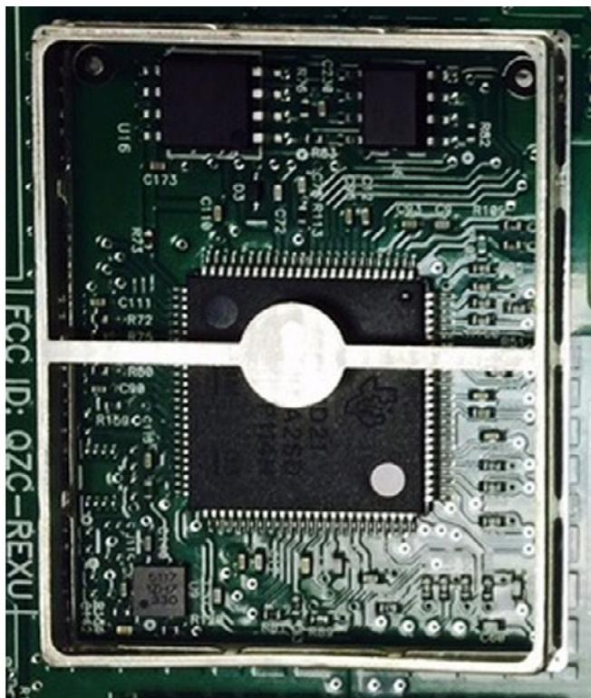
Figure 1: QFP100, 0.5 mm pitch inside of shield—difficult rework project example.
