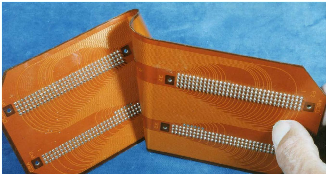
Figure 4: Four connectors: A three-layer FPC with central shield. Terminations are plated through and have soldered connectors.
