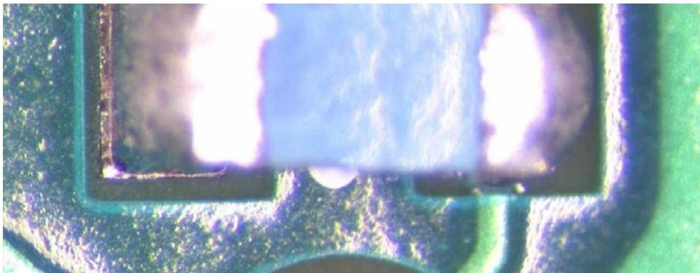
Figure 1: Note area where solder did not completely wet-out.
