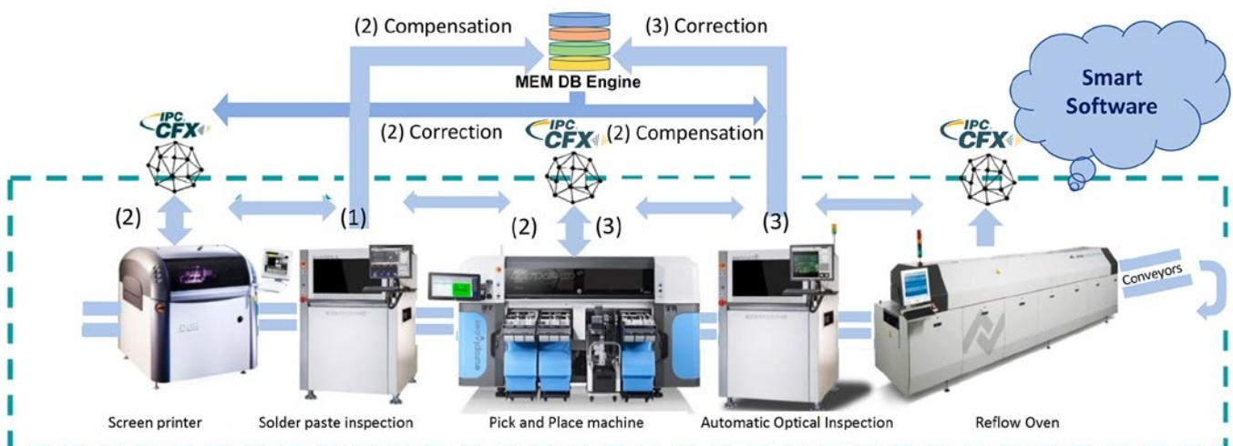
Figure 6: CFX enables assembly machines to talk to each other and pass important data up to management software for higher quality and productivity<sup>4</sup>.
