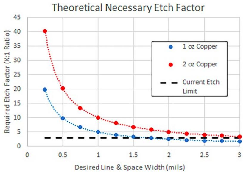
Figure 1: Estimated required etch factor to obtain various feature dimensions on 1-ounce and 2-ounce copper.
