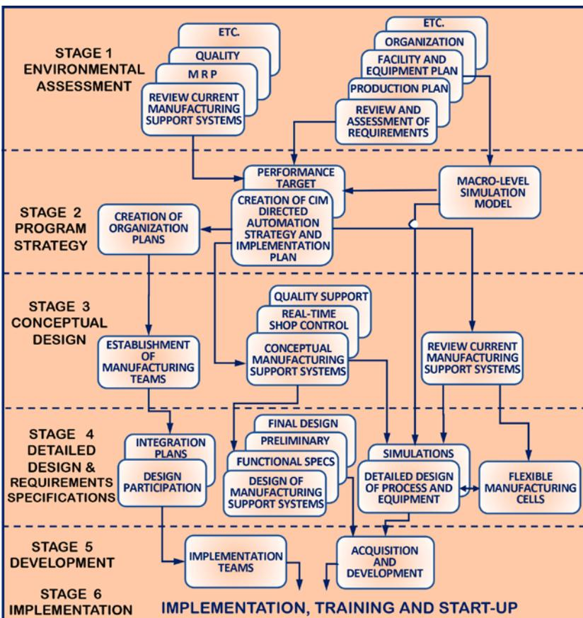
Figure 1: The six stages of planning for a Smart factory<sup>1</sup>.
