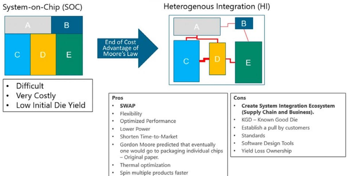
Figure 1: HI using chiplets offers many advantages over conventional SoC, but creating a viable HI ecosystem requires overcoming several challenges.
