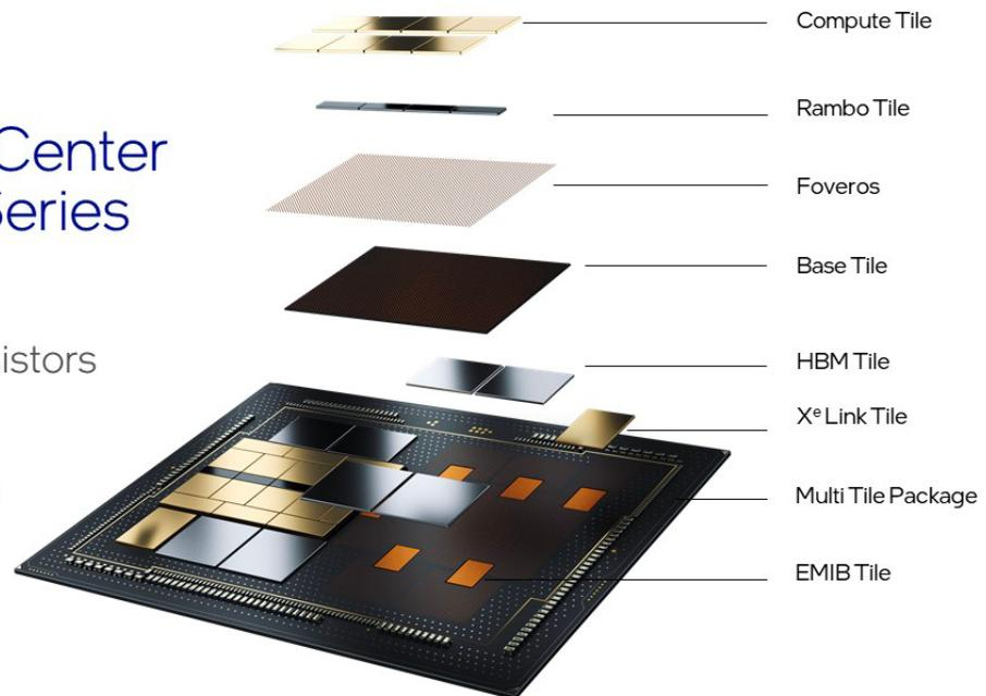
Figure 1: The Intel® Data Center GPU Max Series, an example of a complex advanced package product.
