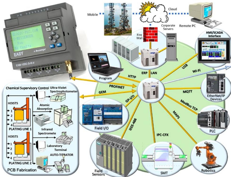
Figure 3: The electronics manufacturing factory floor basically has three standard protocols: PLCs, CFX, and SECS/GEM.
