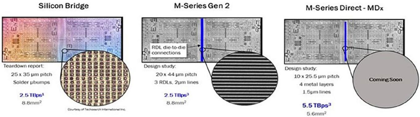
Figure 3: Comparison between heterogeneous integration packages using a) an embedded silicon bridge die; b) M-Series Gen 2; and c) M-Series Direct (MDx).
