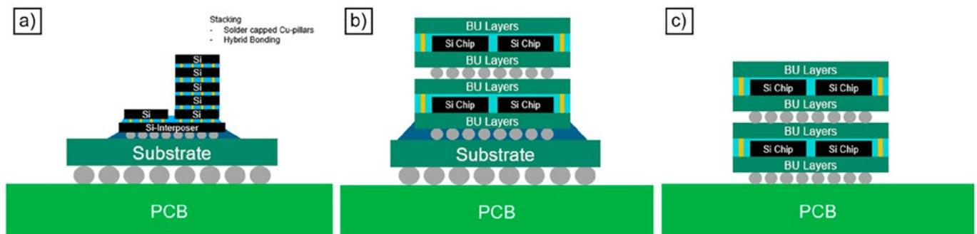
Figure 2: Pathways to advanced heterogeneous integration using a) silicon interposer; b) fan-out wafer level packaging on build-up substrate; and c) fan-out wafer level packaging without substrates.
