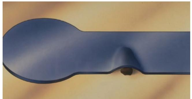
Figure 2: Depression in foil surface with possible resist adhesion issue.
