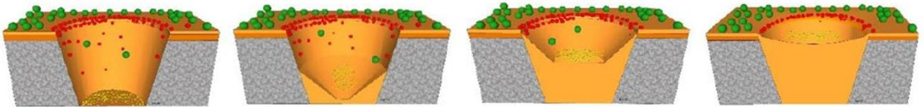
Figure 8: Curvature-enhanced-accelerator-coverage is the result of interactions of the wetter, brightener, and leveler over the course of bottom-up via filling.
