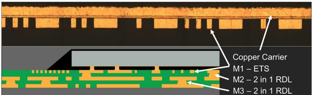
Figure 12: Coreless substrate buildup starts with ETS plating on a removable copper carrier, which is then encased into prepreg and built up with RDL plating.
