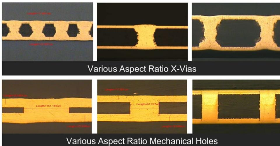
Figure 14: Single-step through-hole filling for the core layer of IC substrates has benefits, ranging from improved thermal management to improved structural stability.
