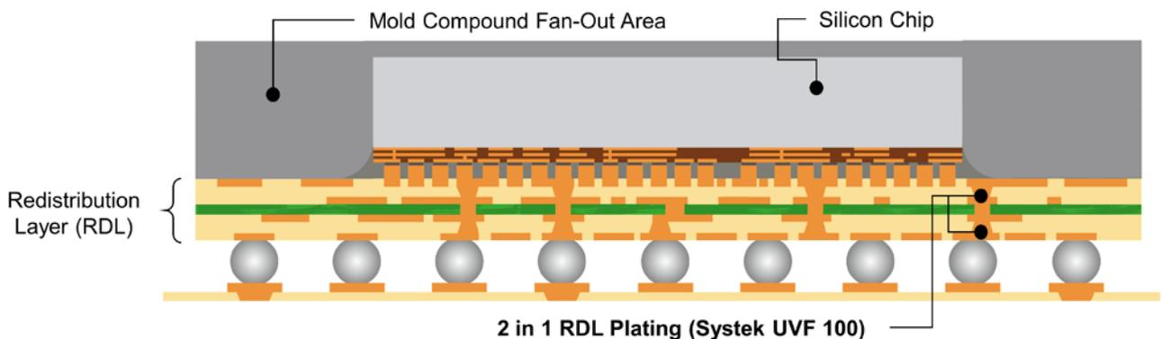
Figure 7: RDL features created with two-in-one via filling and fine-feature plating enable organic substrate buildup.
