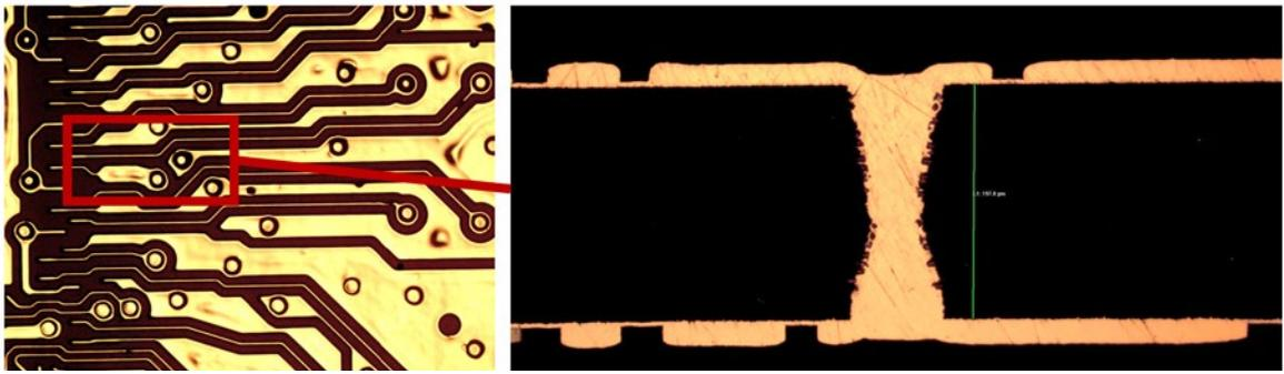
Figure 10: Double-shot laser-drilled core plated with Systek UVF 100 image before final etch.
