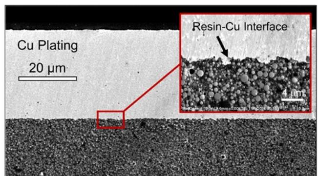
Figure 3: Copper adhesion at the resin-to-copper interface is a critically important metric for the semi-additive seed layer performance.
