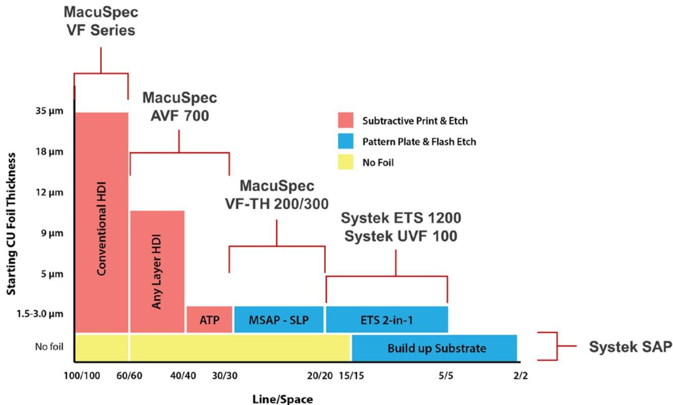
Figure 1: Starting copper foil thickness vs. line/space dimensions for various advanced PCB manufacturing applications and commercial metallization processes associated with them.
