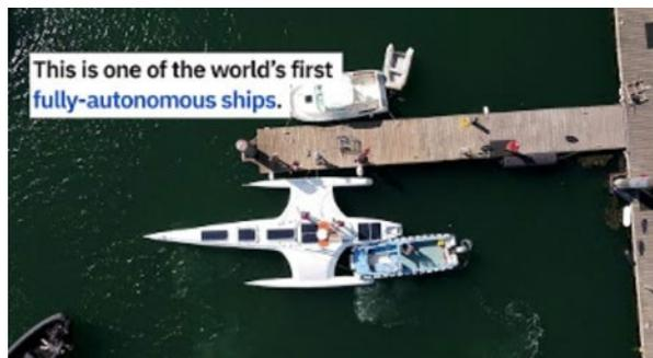
MAS features an AI Captain built by ProMare and IBM developers, which gives MAS the ability to sense, think, and make decisions at sea with no human captain or onboard crew. The new class of marine AI is underpinned by IBM’s latest advanced edge computing systems, automation software, computer vision technology, and Red Hat open-source software.
