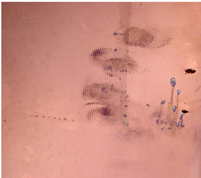
Figure 1: Example of fingerprints on copper.
