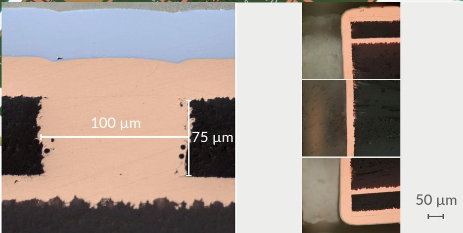
BMV filling with dimple < 5 µm and surface copper 12 µm
