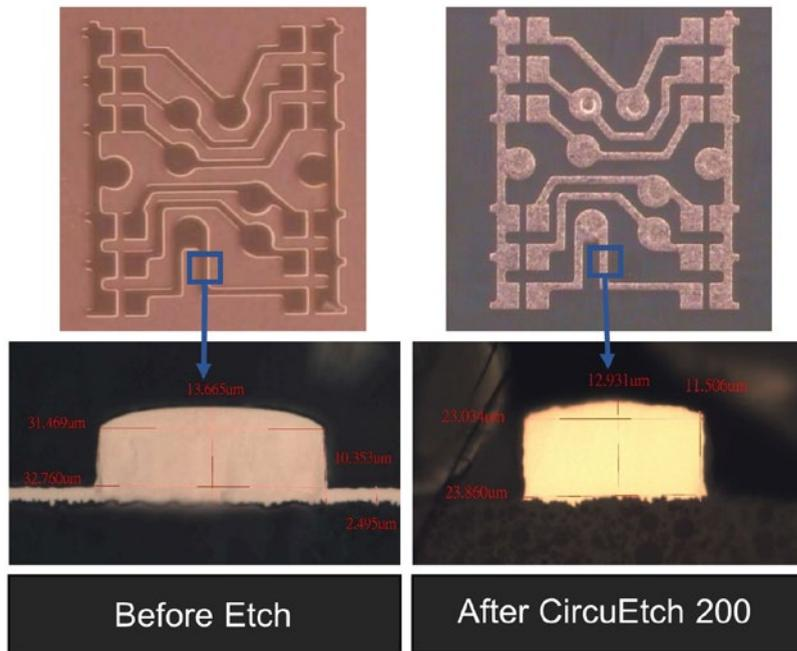
Figure 16: It is critically important that the final etch does not undercut the trace and retains a rectangular cross-section after etching, without removing significant amounts of surface copper.
