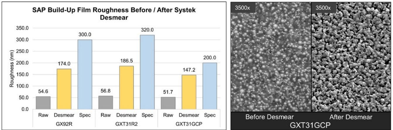
Figure 4: Below-spec roughness of substrate material is a desirable property for substrate electrical performance.
