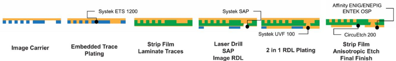
Figure 11: Coreless buildup process for IC substrate.
