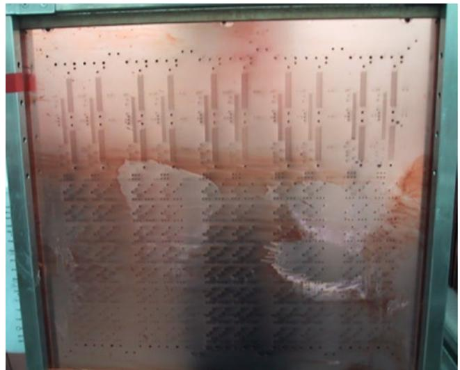
Figure 2: Oxidation. (Source: RBP Chemical Technology)
