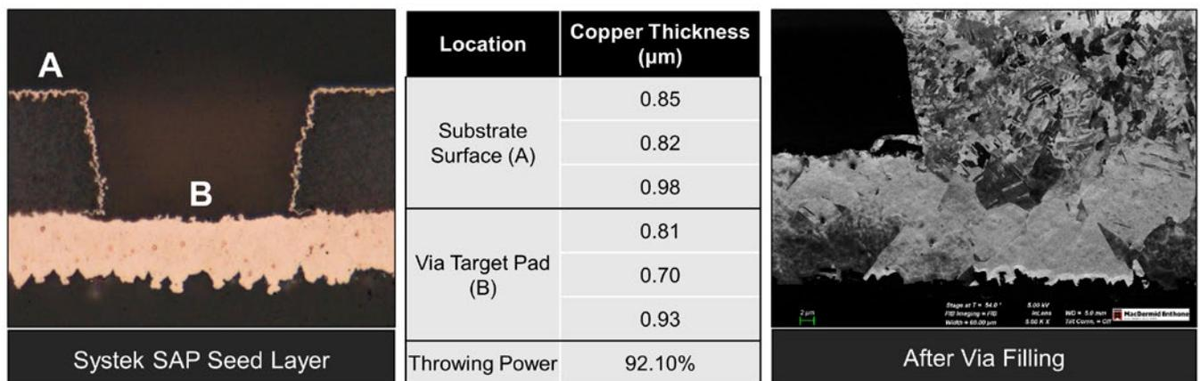
Figure 5: A uniform coating during the SAP seed layer plating is necessary for reliable via filling.
