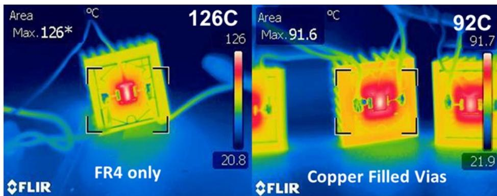
Figure 13: The addition of copper thermal via significantly improves the operating LED junction temperature for longer operating life.
