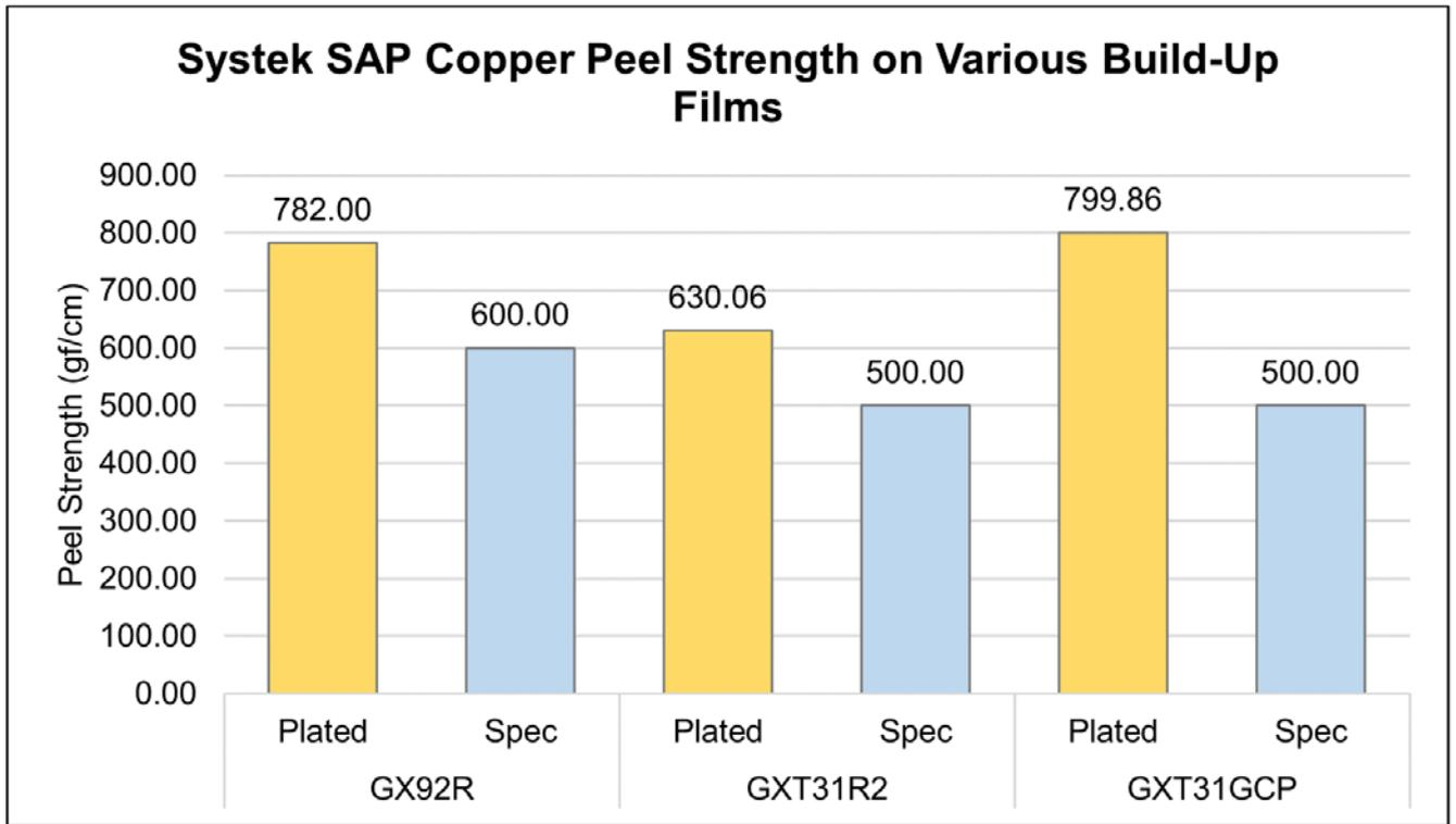
Figure 6: Peel strength of SAP copper plated on multiple ABF substrates.
