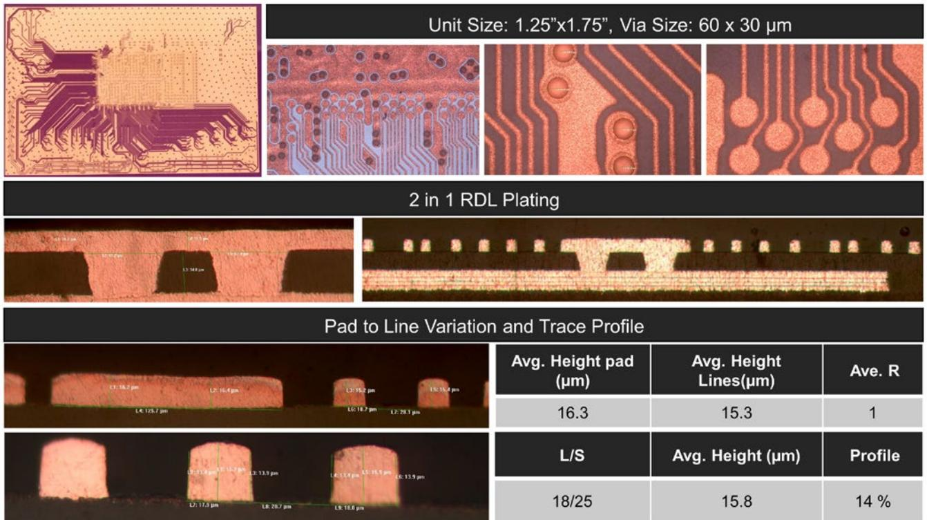
Figure 9: Systek UVF 100 pattern plating on IC substrate RDL.
