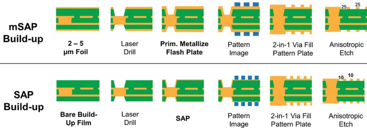
Figure 2: SAP enables finer lines and spaces for IC substrate RDL.
