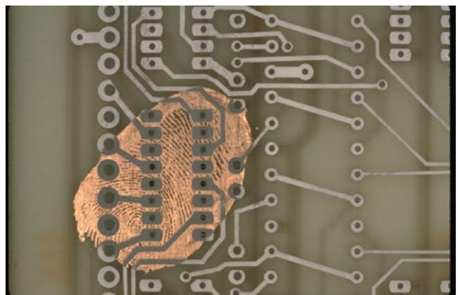
Figure 3: Example of oily fingerprint preventing complete etching of the copper. (Source: RBP Chemical Technology)
