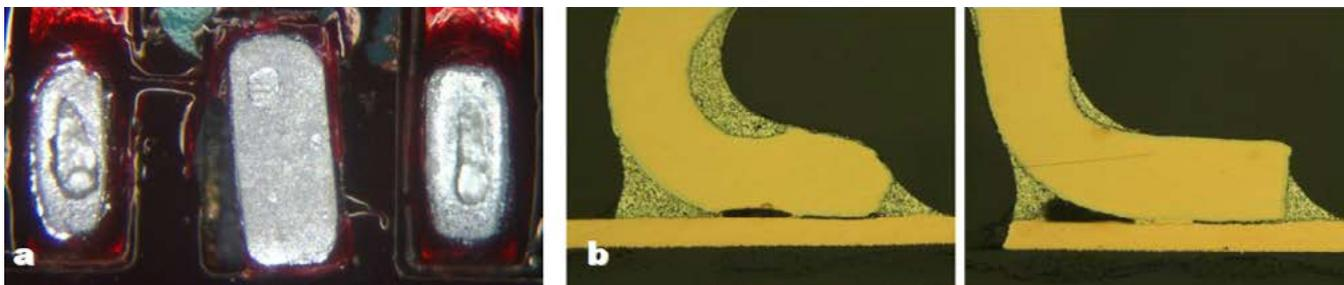
**Figure 8:** Destructive analysis of voided solder joints on SMT array connectors after 1,000 cycles ATC stress testing without failure: a) Case 1 - dye-and-pry analysis (GND, SIG, and GND); b) Case 2 - cross-section analysis of ground and signal leads.
