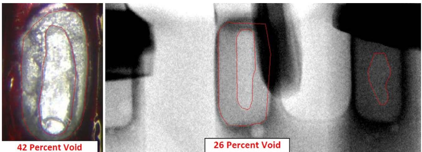
**Figure 7:** Quantitative void assessment examples from two different array connector product applications: a) Dye-and-pry; and, (b) X-ray tomographic measurement.
