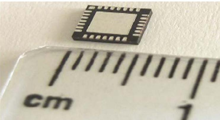
**Figure 1:** A QFN showing its leads and thermal pad.
