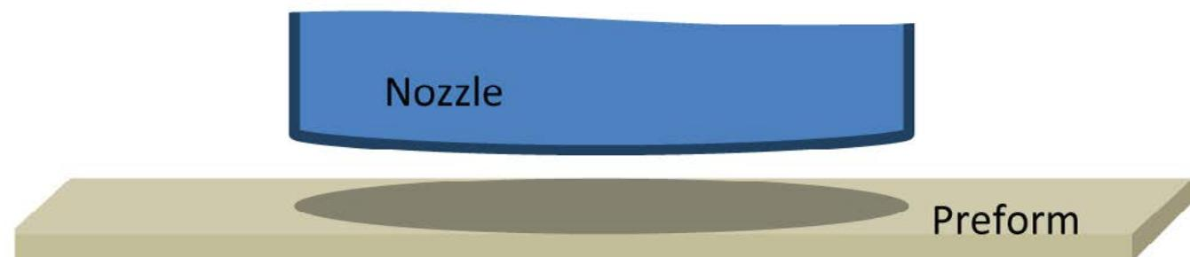
**Figure 5:** The desired relationship between the nozzle and the solder preform.
