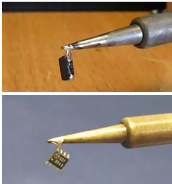
**Figure 1:** Demonstration of the load-carrying capacity of molten solder.
