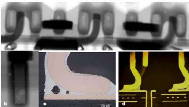
**Figure 1:** Inclusion voids observed in SMT gull wing solder joints with 2D X-ray (a, b) and cross section (c, d).
