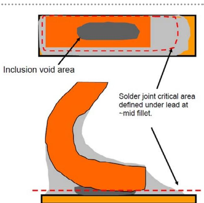
**Figure 6:** Schematic illustration (top and side X-ray view) of void area measurement in a gull wing solder joint relative to the solder joint critical load bearing area.
