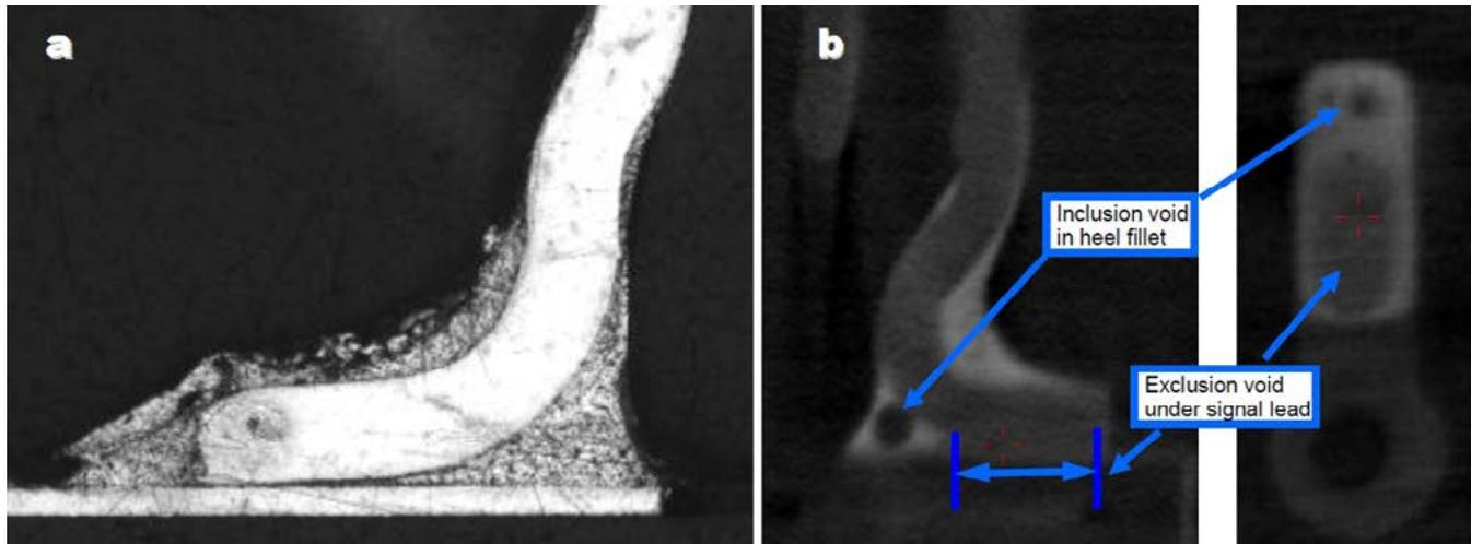
**Figure 3:** Solder exclusion voids found in SMT gull wing solder joints viewed in a.) cross-section and b.) 3D X-ray scans.
