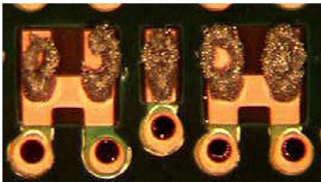
**Figure 2:** Solder paste impression showing solder displaced (squeezed out) from under the highest leads.
