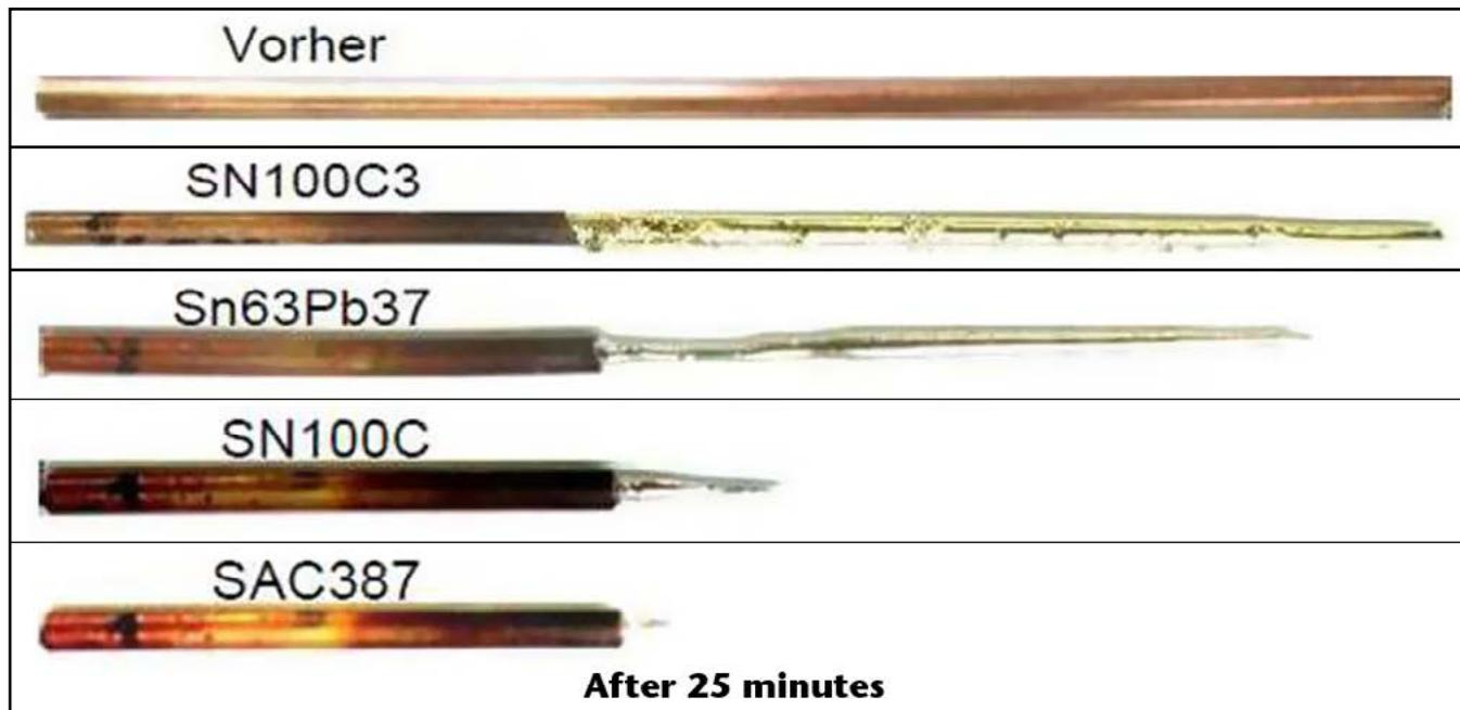
**Figure 2:** Copper wire  $\varnothing$  6 mm, miniwave 360°C, immersion time 40 min/25 min. (Source: Balver Zinn 2012)
