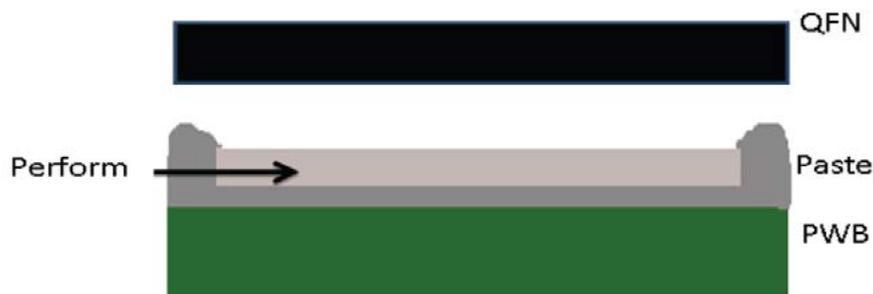
**Figure 4:** Illustration of a rectangular solder preform placed on the solder paste.
