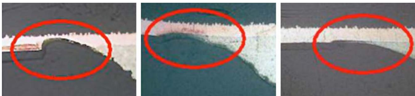
**Figure 7:** Copper alloy with usage of different solder alloys—7a (left), SnAg3,8Cu0,7; 7b (center), SnAg3,5Cu0,5; and 7c (left) SN100C. (Source: Keith Sweatman, Nihon Superior und Balver Zinn 2012)
