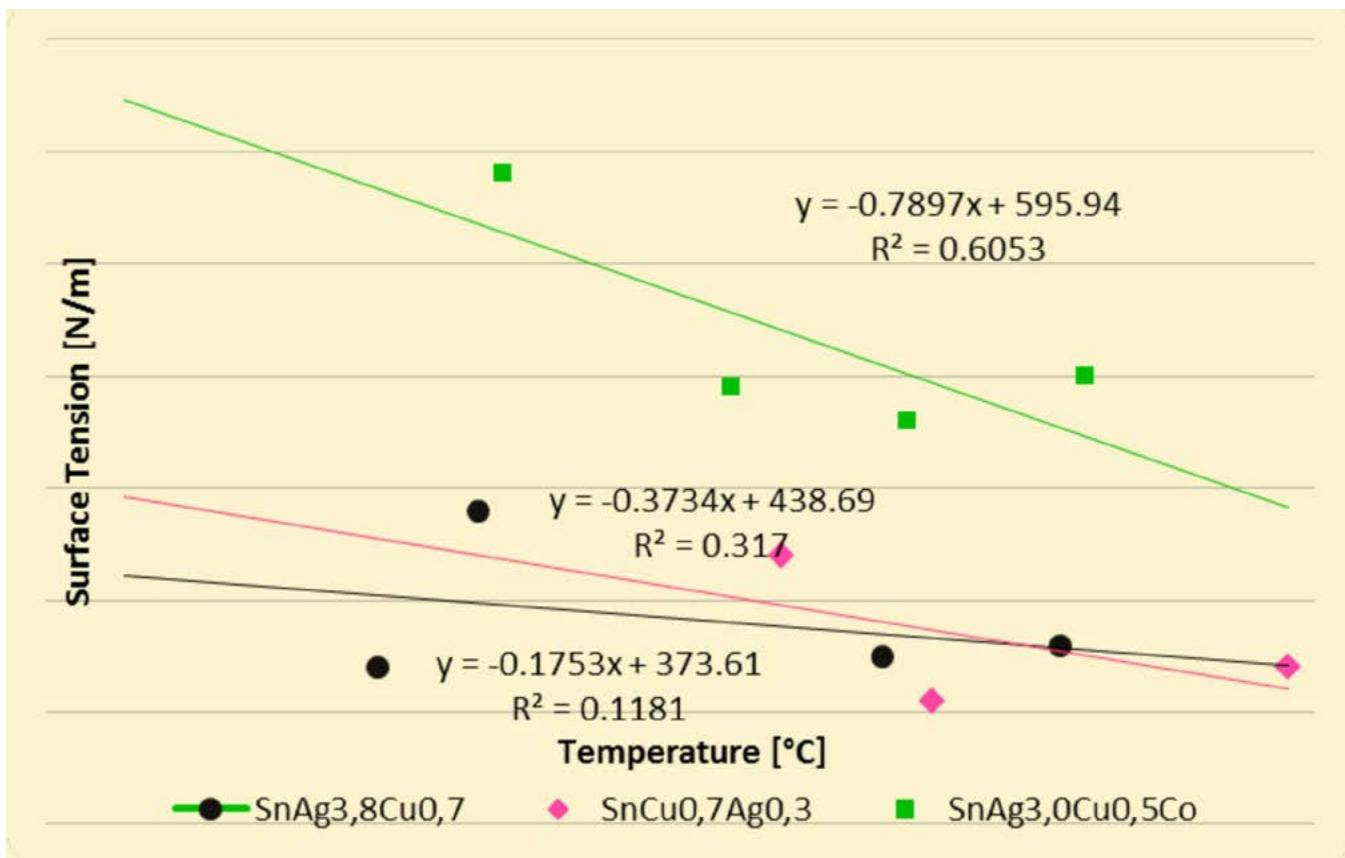
**Figure 10:** Surface tension of SAC solders.
