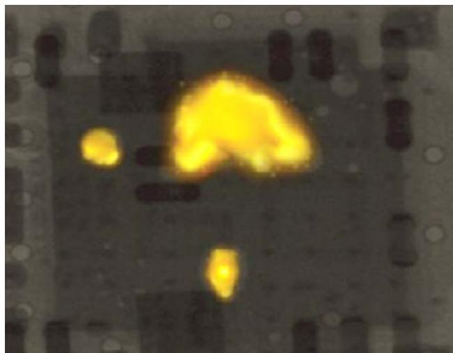
**Figure 3:** Illustration of the result of thermal path obstruction and localized heating.
