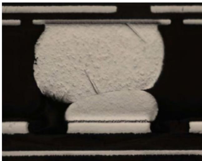
Figure 10: Typical HIP issue when using too long of a soak time and too high of a soak temperature. This issue could pass a functional test and end up as a field return.
