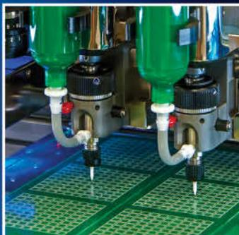
Dual-valve capabilities: dual-action or dual simultaneous dispensing
