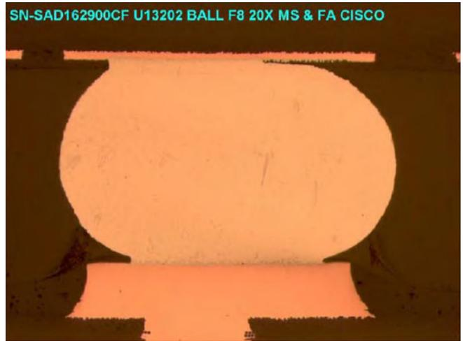
Figure 5: Partial solder separation.
