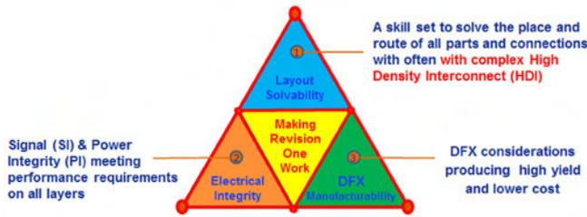
Figure 1: Per IPC-2200 series: three perspectives for PCB design layout success.
