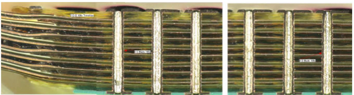
Figure 7: Microsection of flex/rigid transition zone and rigid section (with vias).
