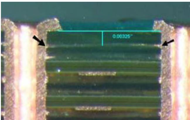
Figure 17: Microsection of CAF coupon fail site.
