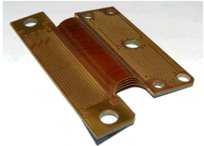
Figure 22: Rigid-flex with LGA contacts shown.
