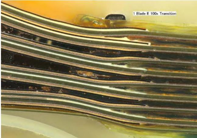
Figure 8: Microsection of flex/rigid transition zone.
