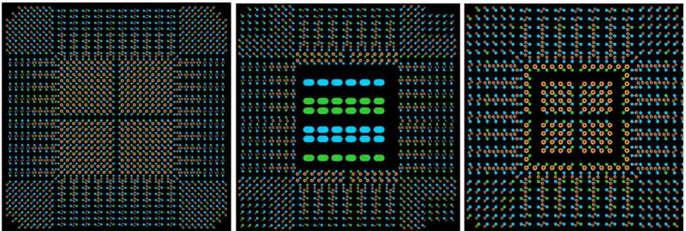
Figure 6: Example for a Virtex 5, 1760 pin FPGA. Three alternative surface breakout using ‘swing vias’<sup>[7]</sup>.
