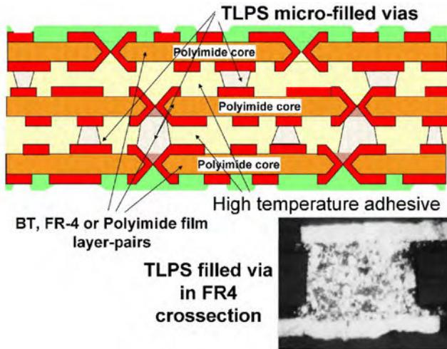
Figure 10: The co-lamination (OrmeLink) multilayer structure<sup>[8]</sup>.
