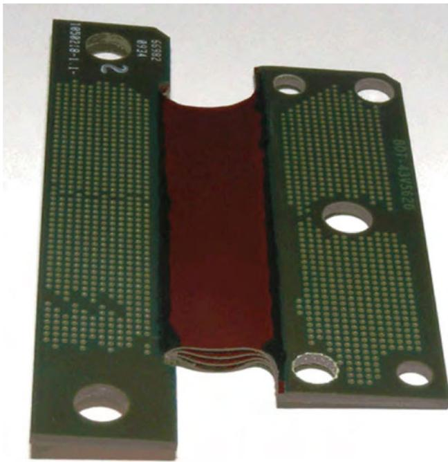
Figure 23: Rigid-flex with backside shown.
