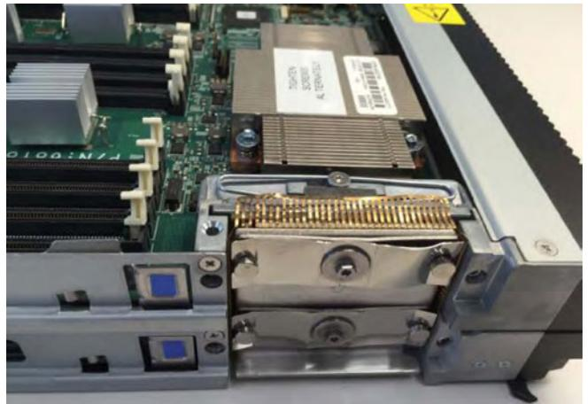
Figure 28: Two-blade system with scalability card and hardware installed.
