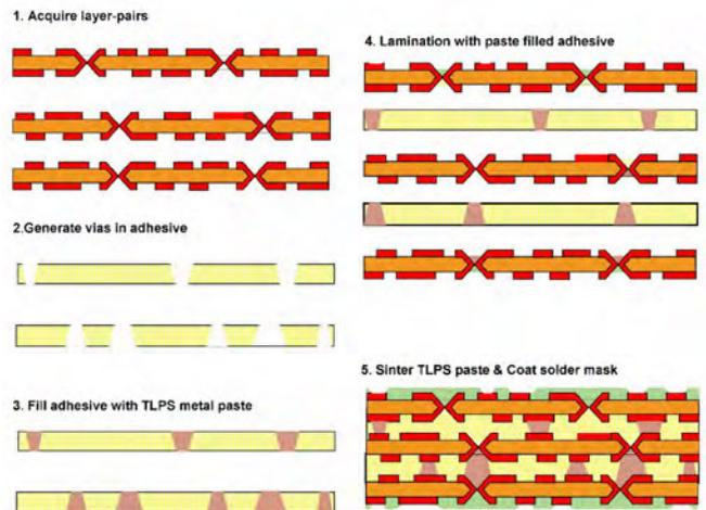
Figure 12: The OrmeLink multilayer substrate fabrication process<sup>[8]</sup>.
