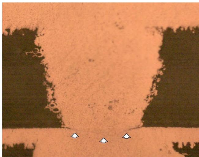
Figure 7: Separation in a microvia.
