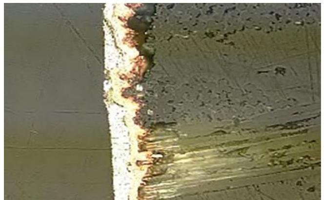
Figure 2: Rough hole walls due to less than optimum drilling (Source: IPC photo archive).
