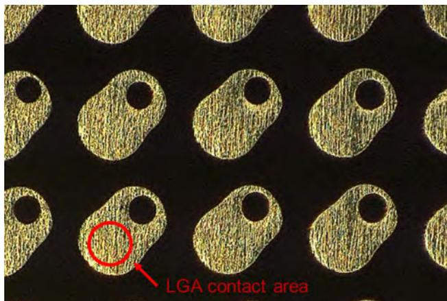
Figure 14: Via and LGA pad structure.
