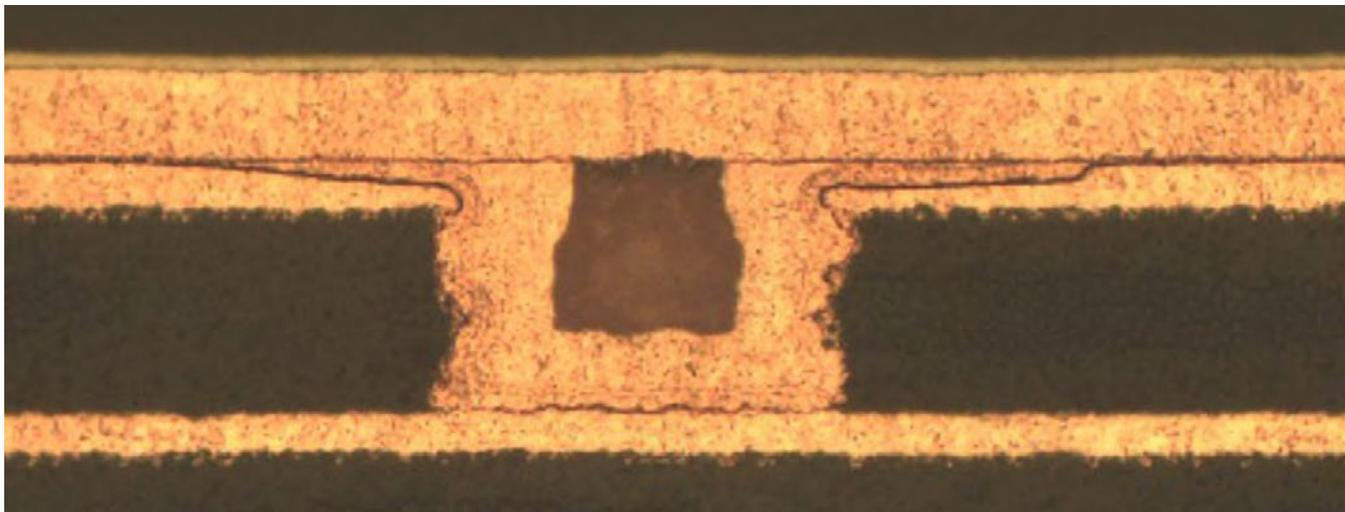
Figure 5: Filled microvia.
