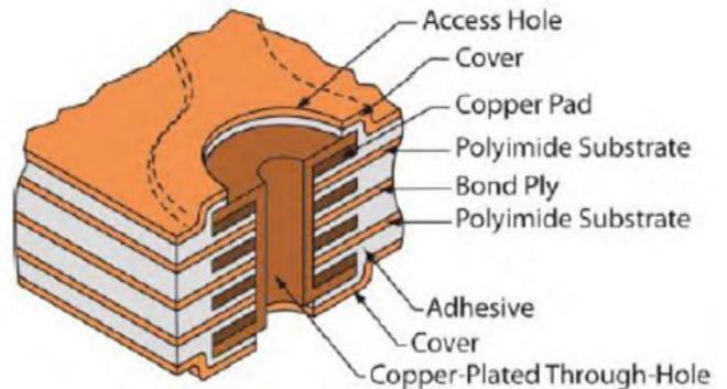
Figure 2: Typical type 3 construction.
