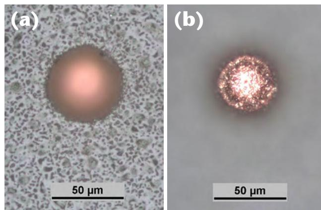
Figure 3: Top ABF surface (a) and bottom copper surface (b) views of a blind microvia drilled with a pulsed UV laser at high PRF with 3,300 holes/sec throughput.
