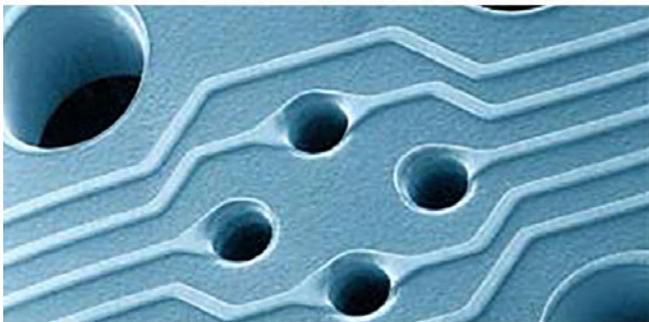
Figure 2: Typical landless vias on a Japanese multilayer from around 1985<sup>[1]</sup>.
