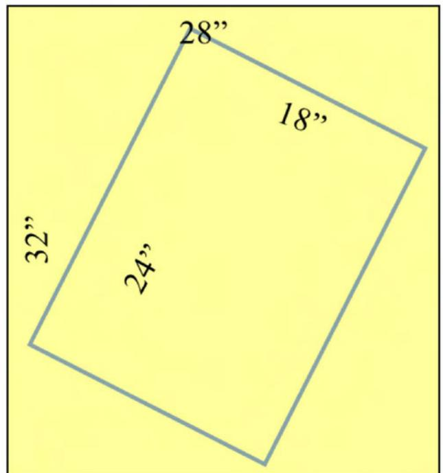
Figure 20: Prepreg panel utilization with rotation.
