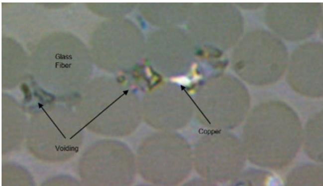
Figure 18: Orthogonal microsection of CAF coupon fail site.
