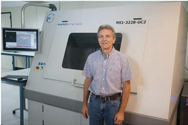
*"More and more our customers are faced with building boards that have multiple microvias that must be carefully controlled and plated with copper. Not having in-house capability to do this, they come to Nova Drilling. Our new Nano System UV/CO2 laser system with its software enhanced trepanning functions allows us to drill vias as small as 25 microns with side walls and bottom surface ideal for plating."*
