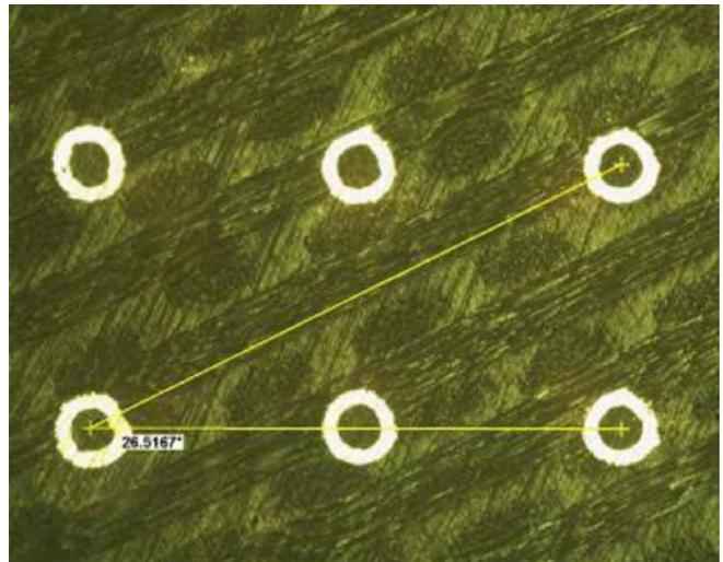
Figure 19: Confirmation of prepreg rotation.
