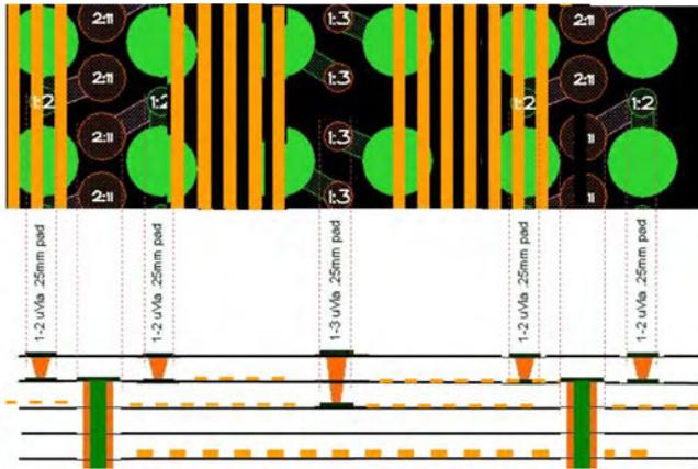
Figure 8: Close-up of Virtex 5 breakout of Figure 7<sup>[7]</sup>.
