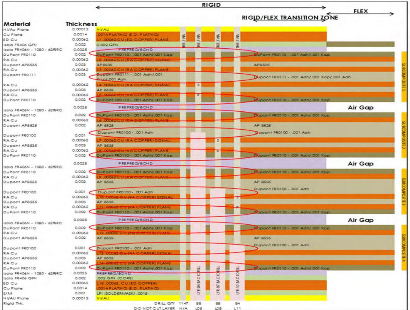
Figure 6: Alternate stack-up without cutback coverlay/acrylic bonding film (not used).
