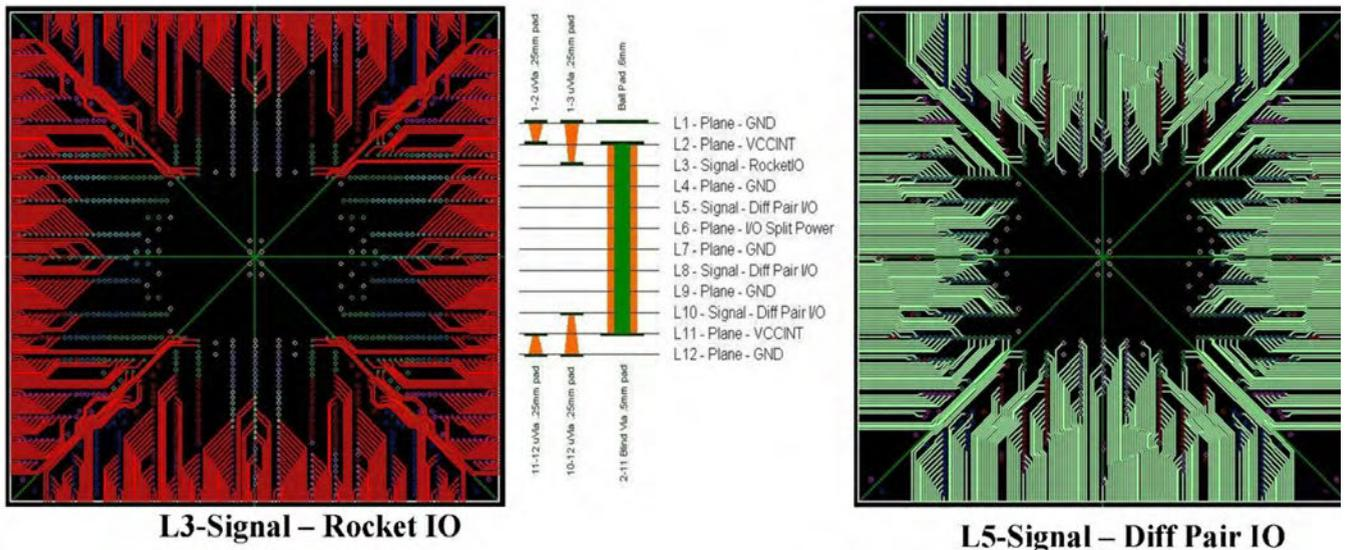
Figure 7: Example for Virtex 5, 1760 pin FPGA, Layer 3 and Layer 5 breakout boulevard routing with stackup view<sup>[7]</sup>.
