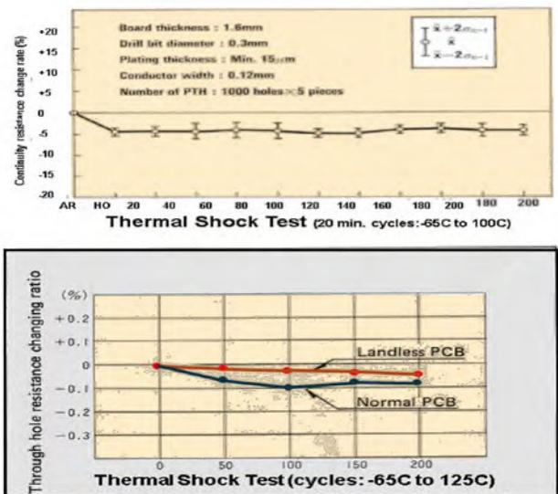
Figure 1: Reliability data from NEC on their landless via fabrication process<sup>[1]</sup>.
