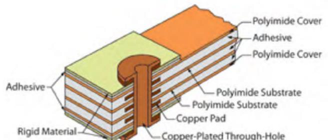
Figure 3: Typical type 4 rigid-flex construction.
