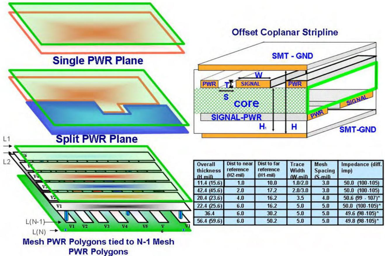
Figure 13: Single (a) and split plane (b) PDN for multilayers with (c) the power mesh architecture modeled as (d) offset coplanar stripline and (e) impedances of this structure<sup>[9]</sup>.
