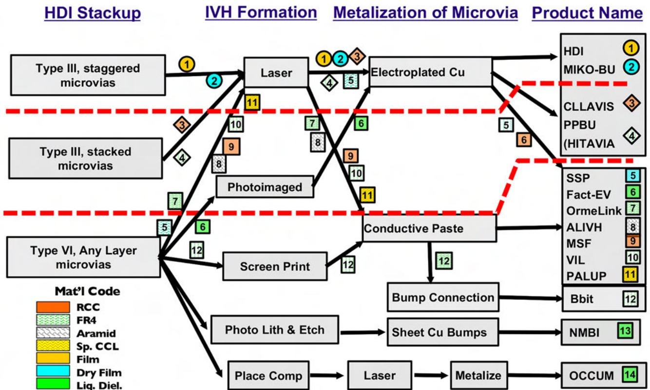
Figure 9: The HDI technologies in use today are made up of four important factors: The microvia stack-up architecture, the dielectric materials, the methods of IVH formation, and the method of metallization of those z-axis via connections. In recent years, 14 different HDI processes have been developed<sup>[8]</sup>.
